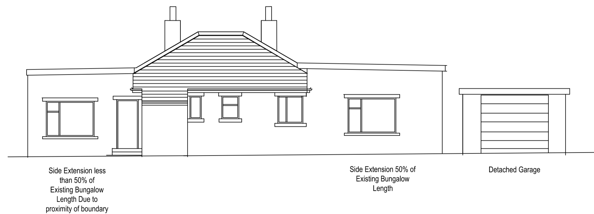
NW ELEVATION (EXISTING WITH PD EXTENSIONS)
