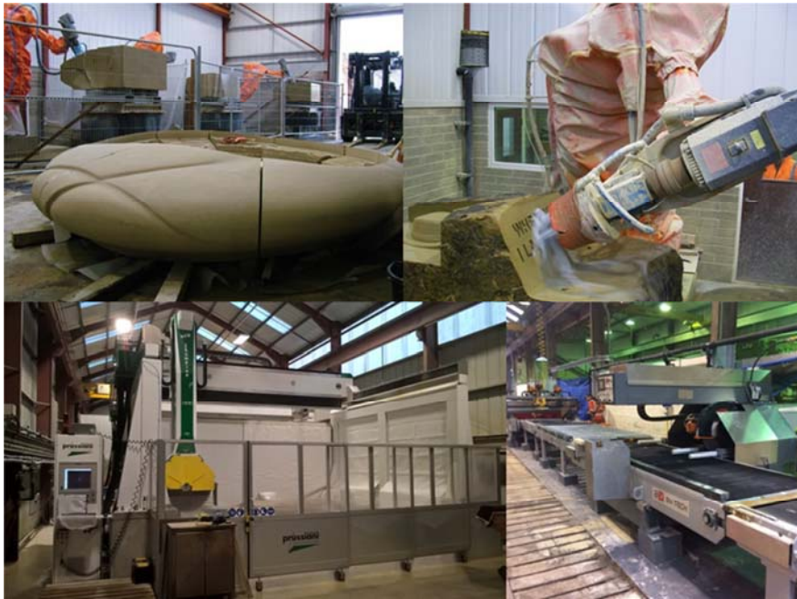
Figure 4.1 Robotic masonry and stone saw technology at Crosland Hill
