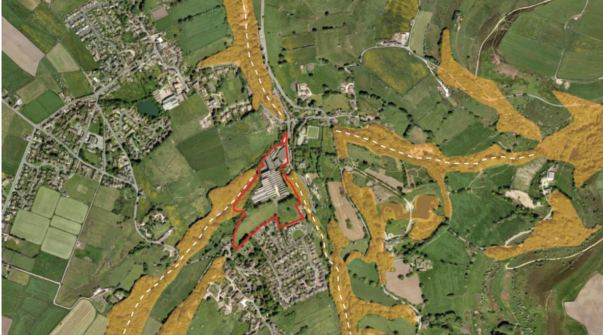
Figure 2 Analysis of wildlife corridors (white dashed lines) and higher value habitat (orange) in relation to the Site.
