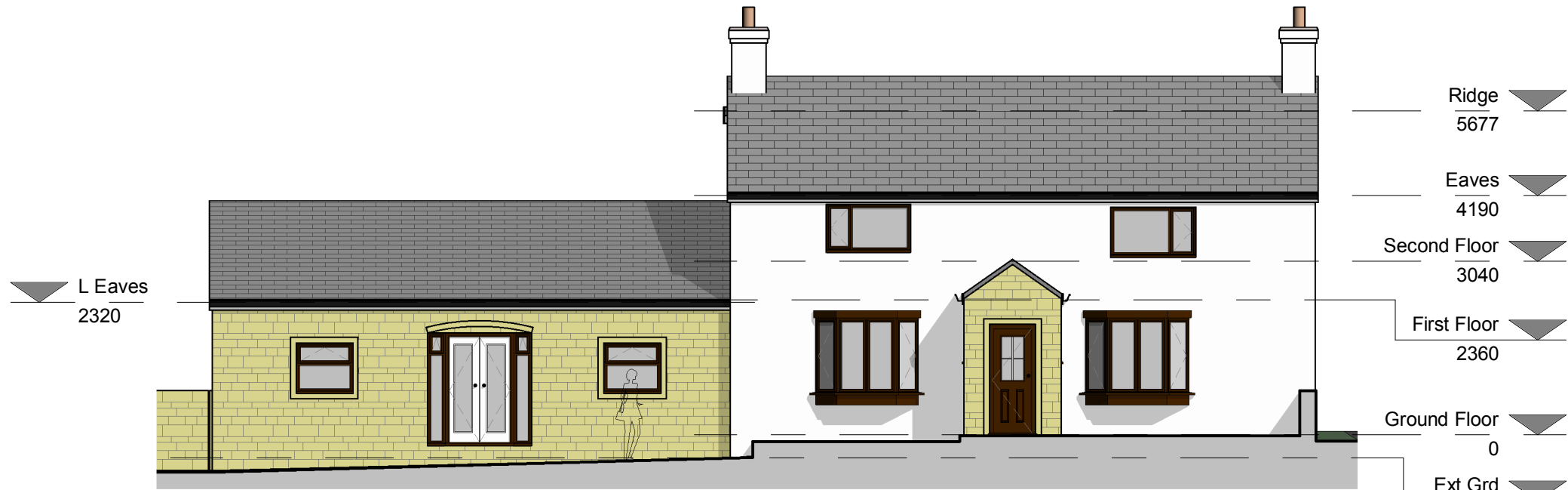
Front Elevation (SW Facing) 1 : 100
