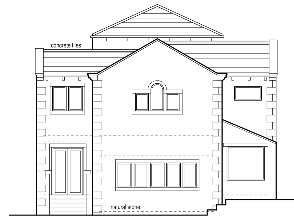
Existing rear elevation (1:100)
