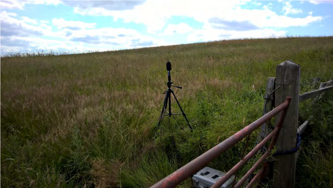
Figure B.3: Sound level meter on a tripod on west boundary of residential zone, along Cliff Hollins Lane
