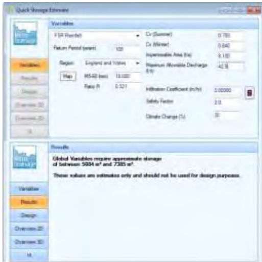
Figure 9. Microdrainage Quick Storage Estimate Attenuation Assessment – Residential Area
