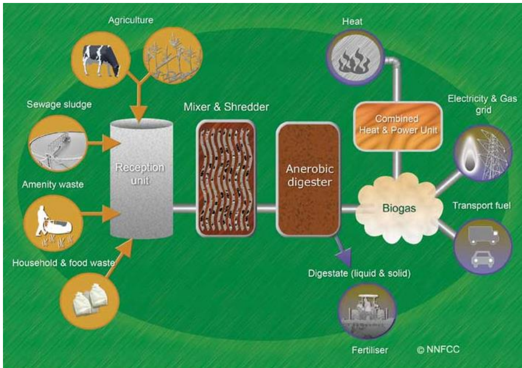
Figure 4-2: Anaerobic Digester System (from www.biogas-info.co.uk)
