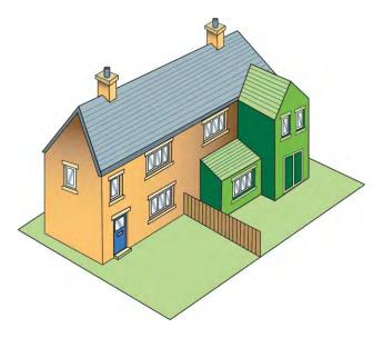
Figure 18: Acceptable part two storey, part single storey rear extension which does not affect the neighbouring property.
