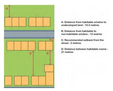
Figure 7: Minimum recommended separation distances.
