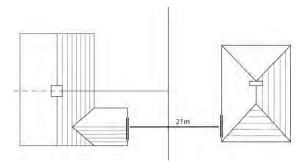
Figure 6: 21m recommended distance between habitable rooms.
