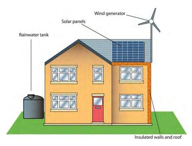
Figure 11: Illustrative example of an extension achieving energy efficiency methods though the use of climate mitigation and adaptation strategies.
