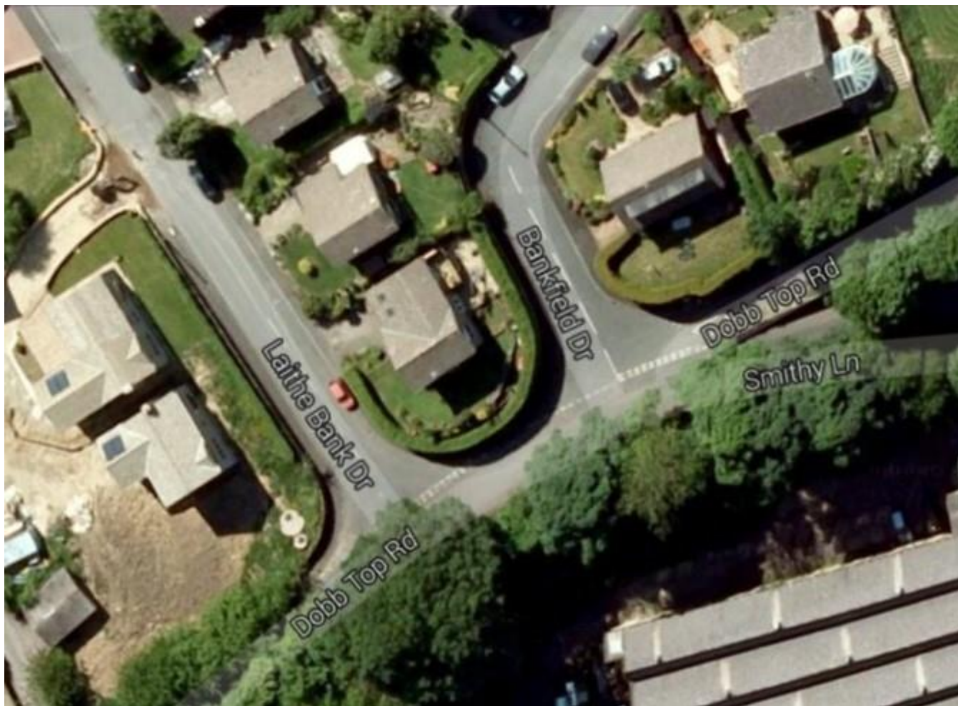
Photo 1 shows the road layout at the bottom of Bankfield Drive and Laithe Bank Drive. The high wall which blocks visibility when pulling out of Bankfield Drive is shown on the right under the Dobb Top Rd sign. Smithy Lane is only 4.7 metres wide wall to wall and traffic has to give way to single file.
