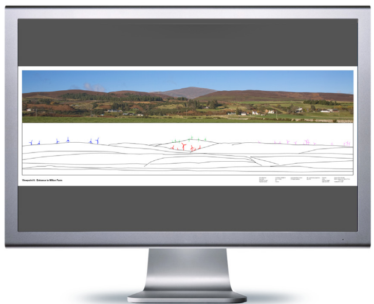
Fig. 17. When the 820mm wide A1 panorama is viewed through an ePlanning portal where it is reduced down to the width of a computer screen, our perception of turbine scale is under-represented by up to a factor of four*.
