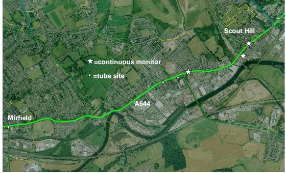
The location of the air monitoring equipment is shown below. The continuous monitors measure oxides of nitrogen (NOx) and small particulates (PM10)
