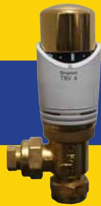
TRVs monitor the air temperature around them and regulate the flow of hot water entering the radiators to keep a set temperature in a room. They allow you to set lower temperatures in some rooms than in others, and to turn off the heating in rooms that aren't used.
