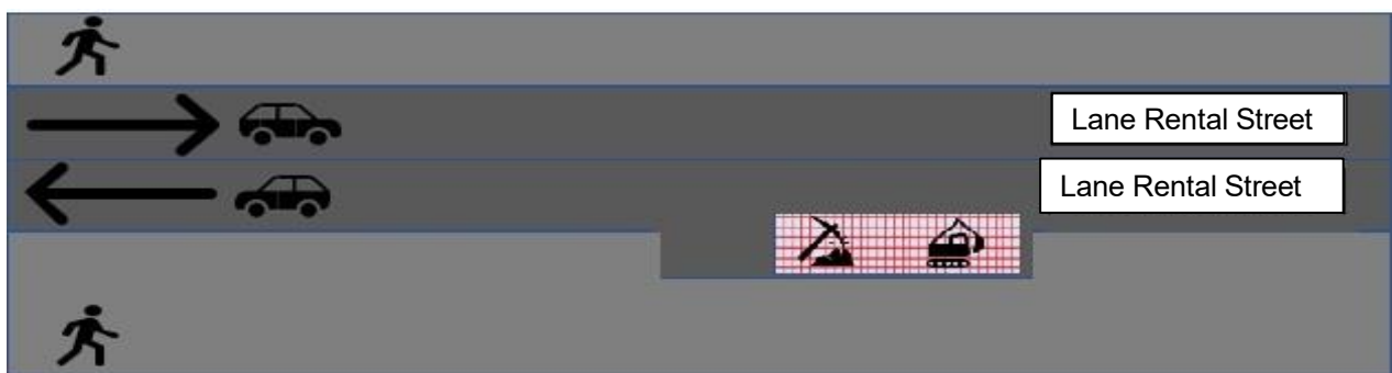
Figure 15: Partial or semi recessed road space.
