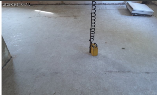
Sampling pump (sample ref: 26/8/A/19/MH5)
