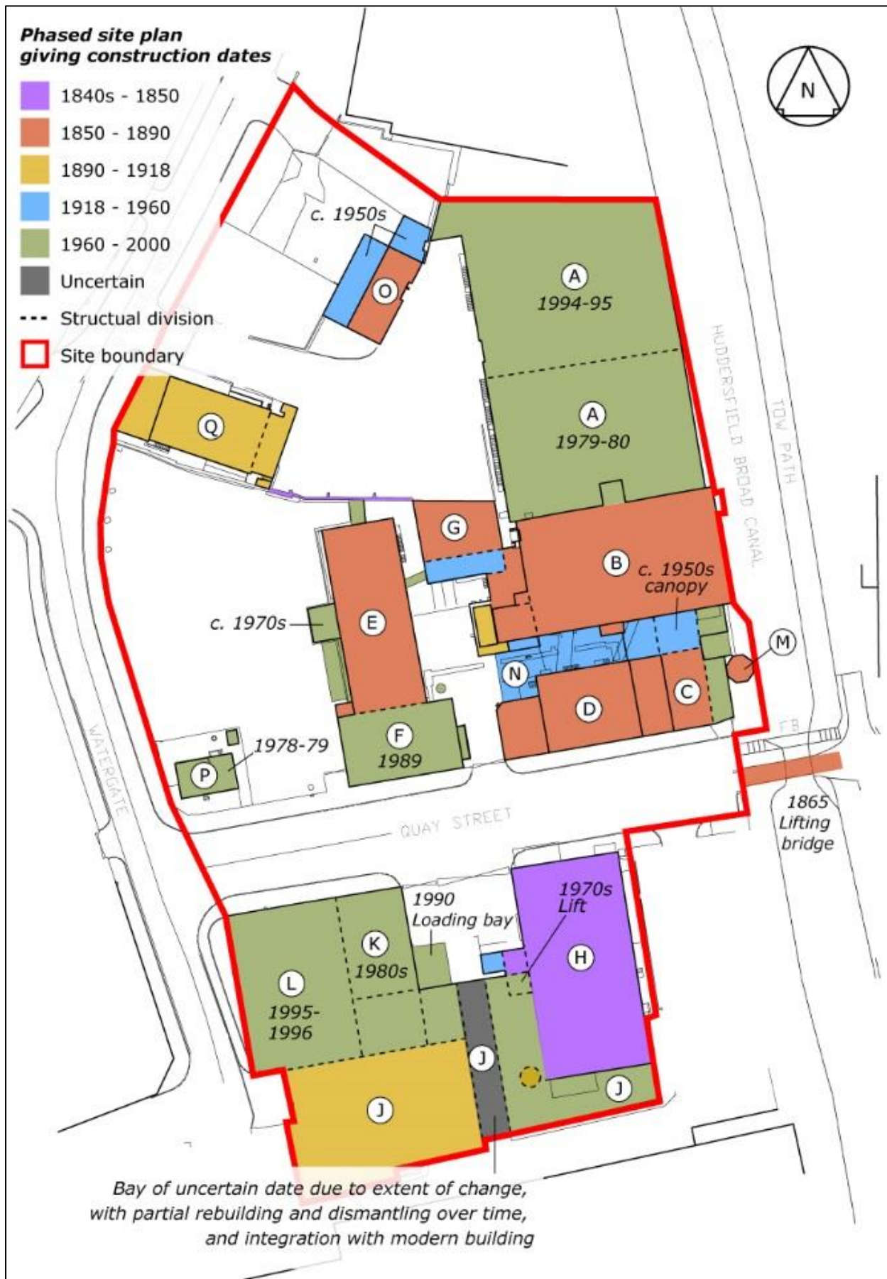
Figure 10: Phased plan of the buildings and structures across the mill complex
