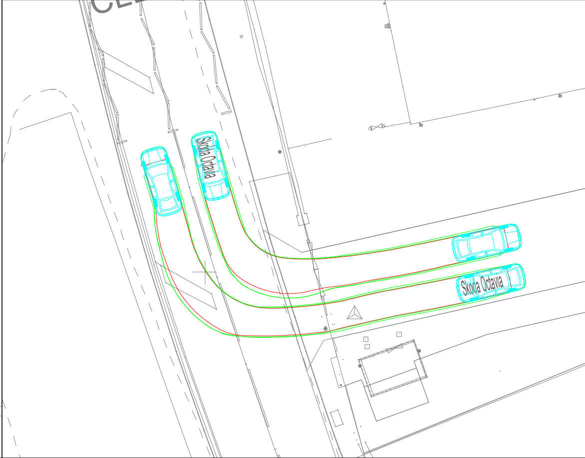
ACCESS SWEEP PATH LEFT IN RIGHT OUT (1:250)
