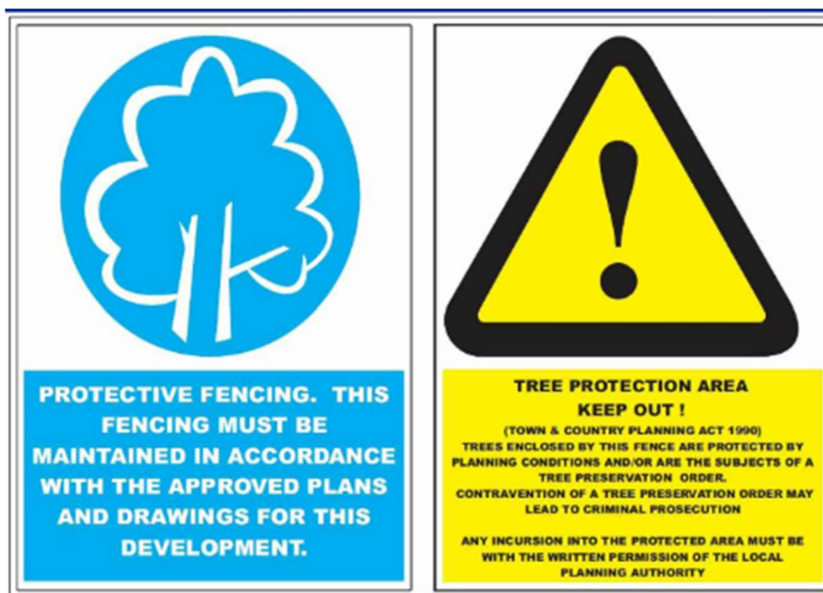
Figure 4 Typical tree protection fencing signage
