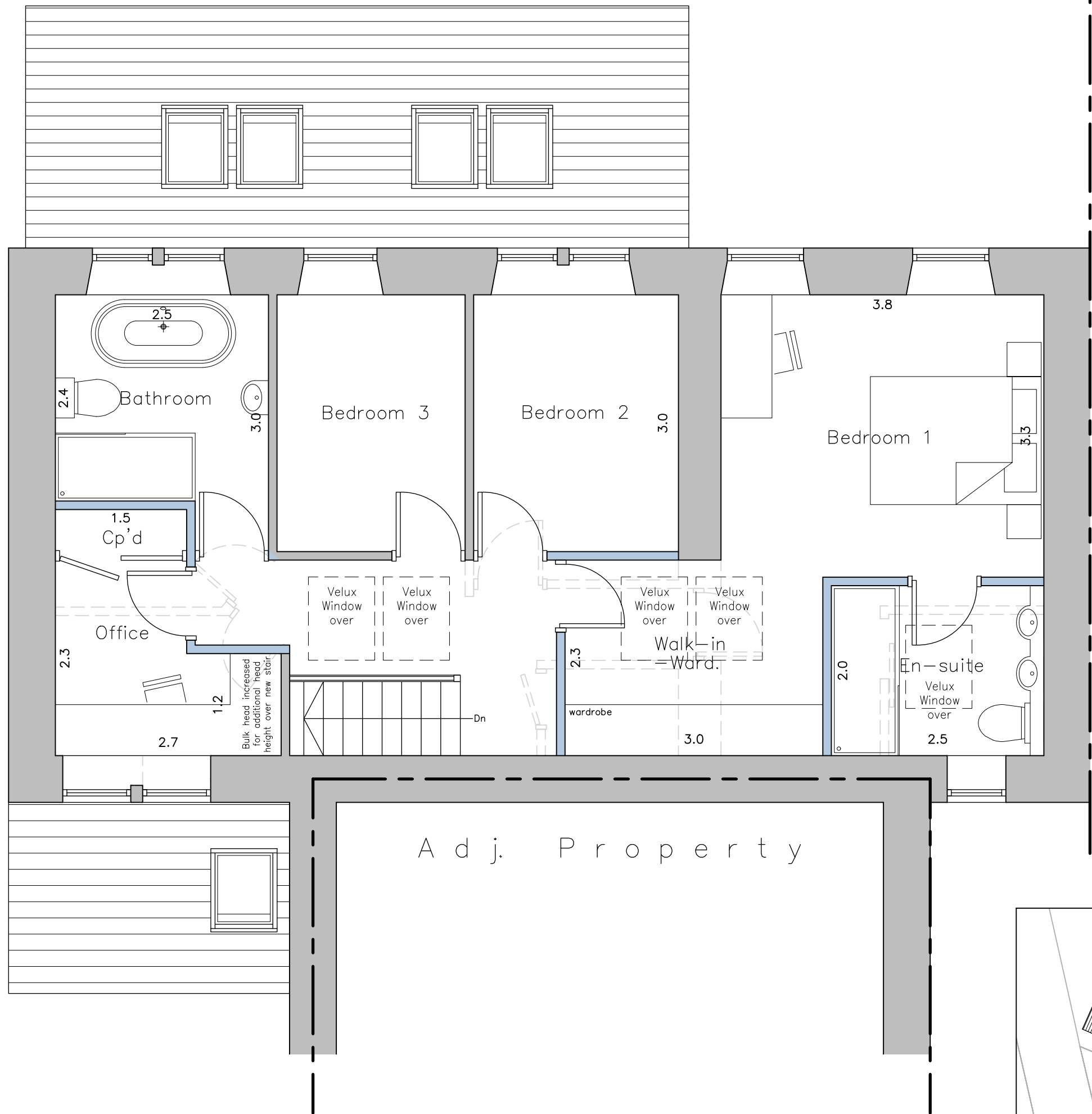
Proposed First Floor Layout Scale 1:50
