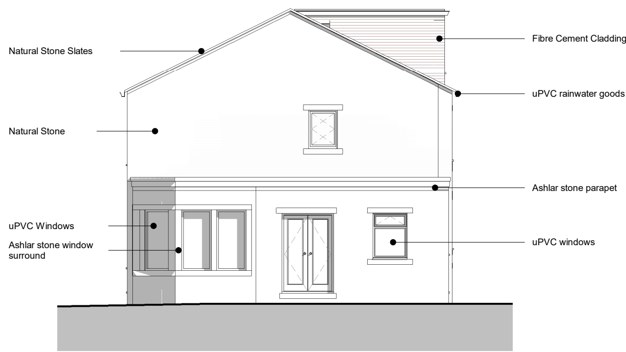
E2 Proposed West Elevation 1 : 100
