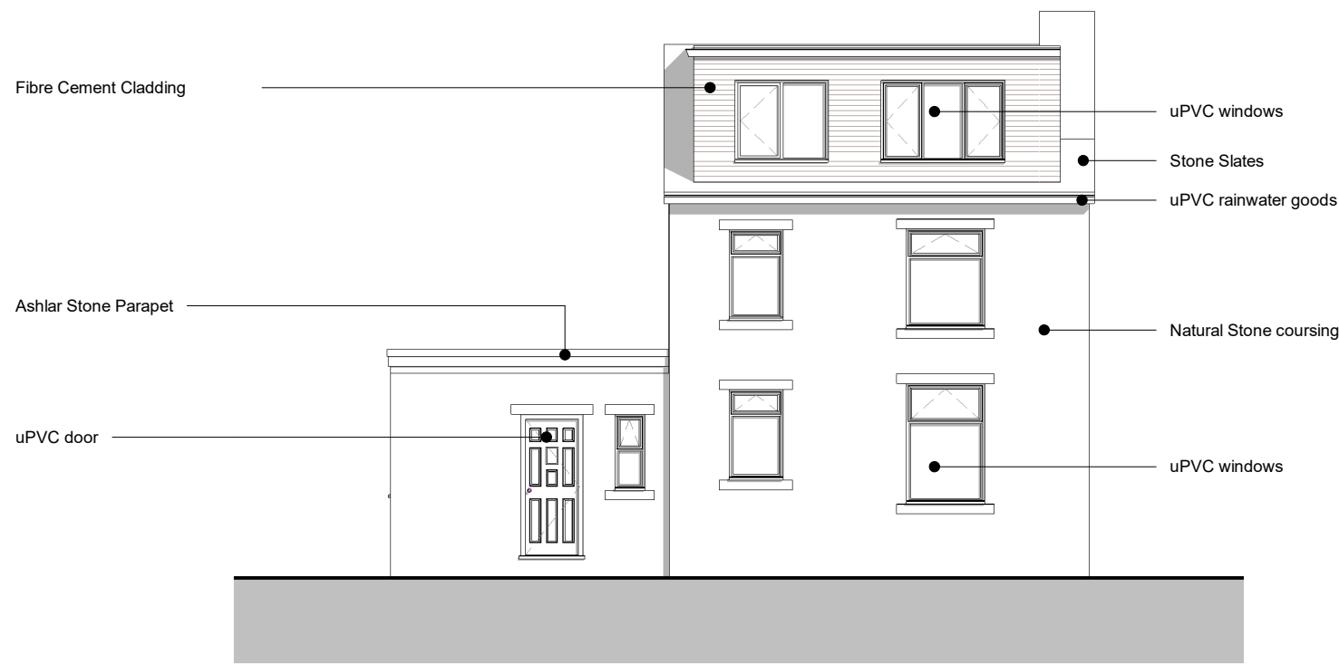
E3 Proposed South Elevation 1 : 100
