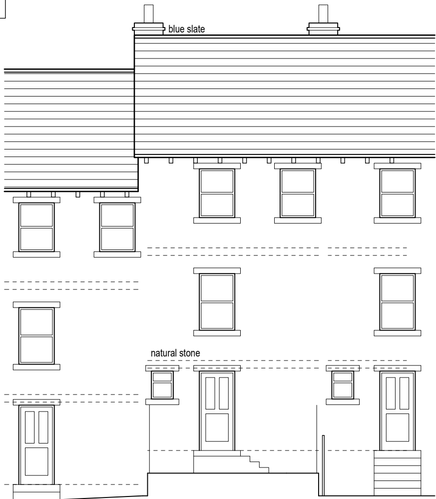
Proposed rear/west facing elevation from patio (1:100)
