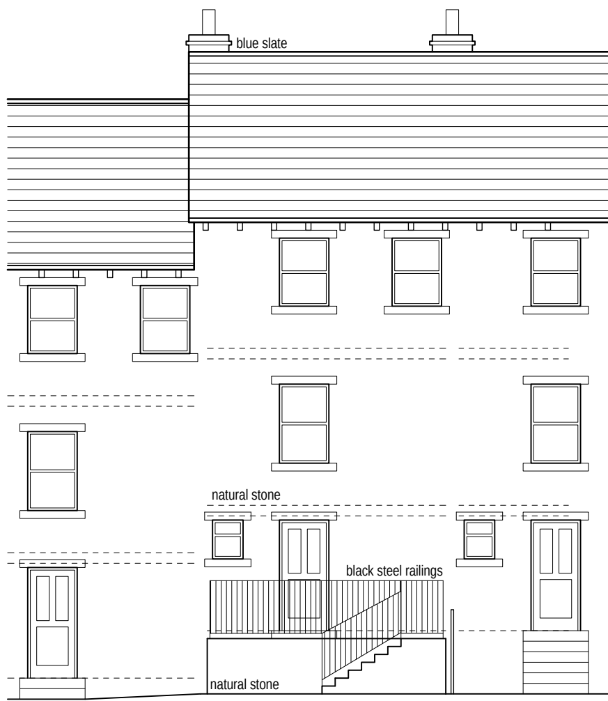
Existing rear/west facing elevation (1:100)
