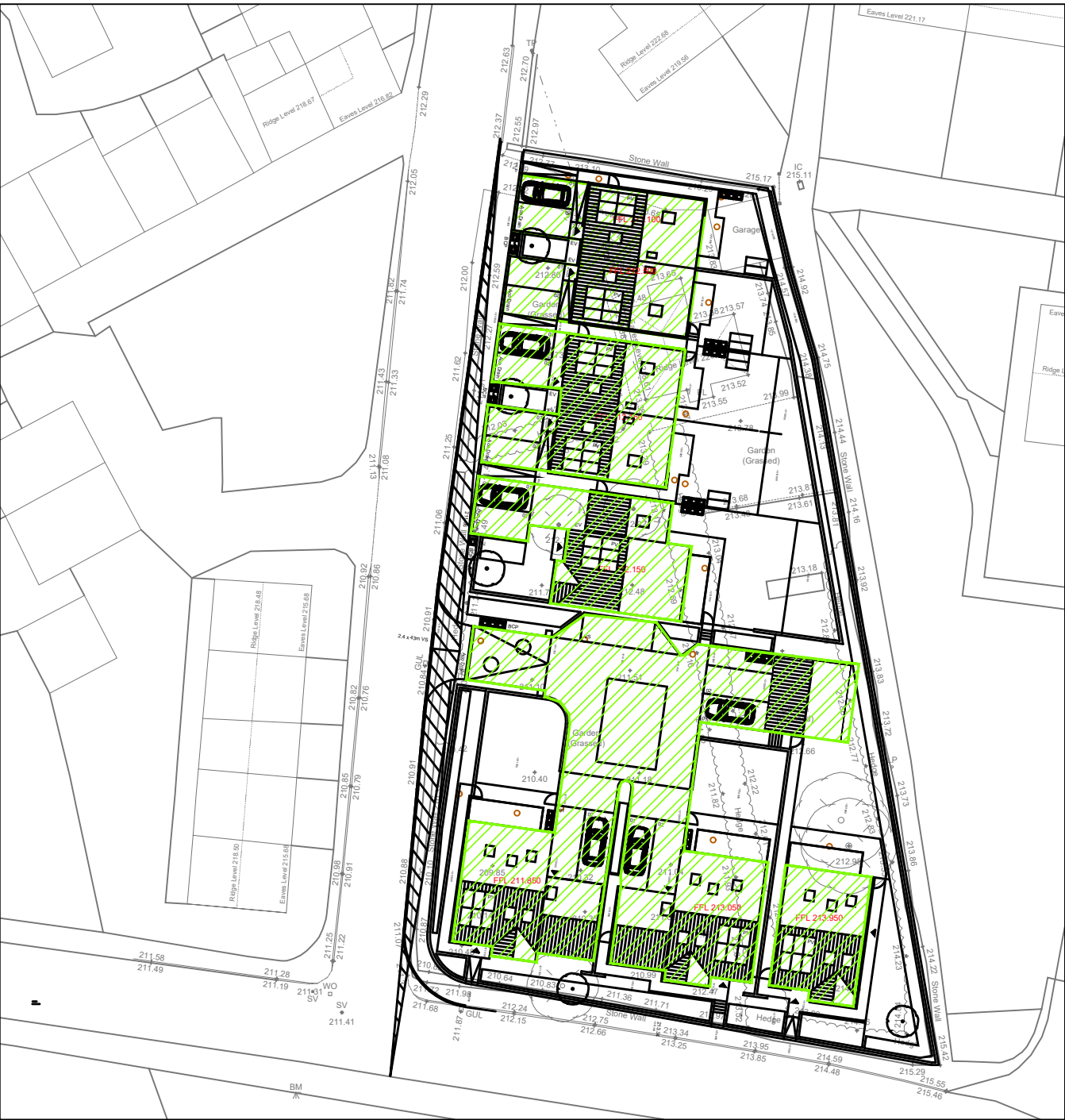
Proposed Impermeable Area Plan 1,200m2 - Scale (1:500)
