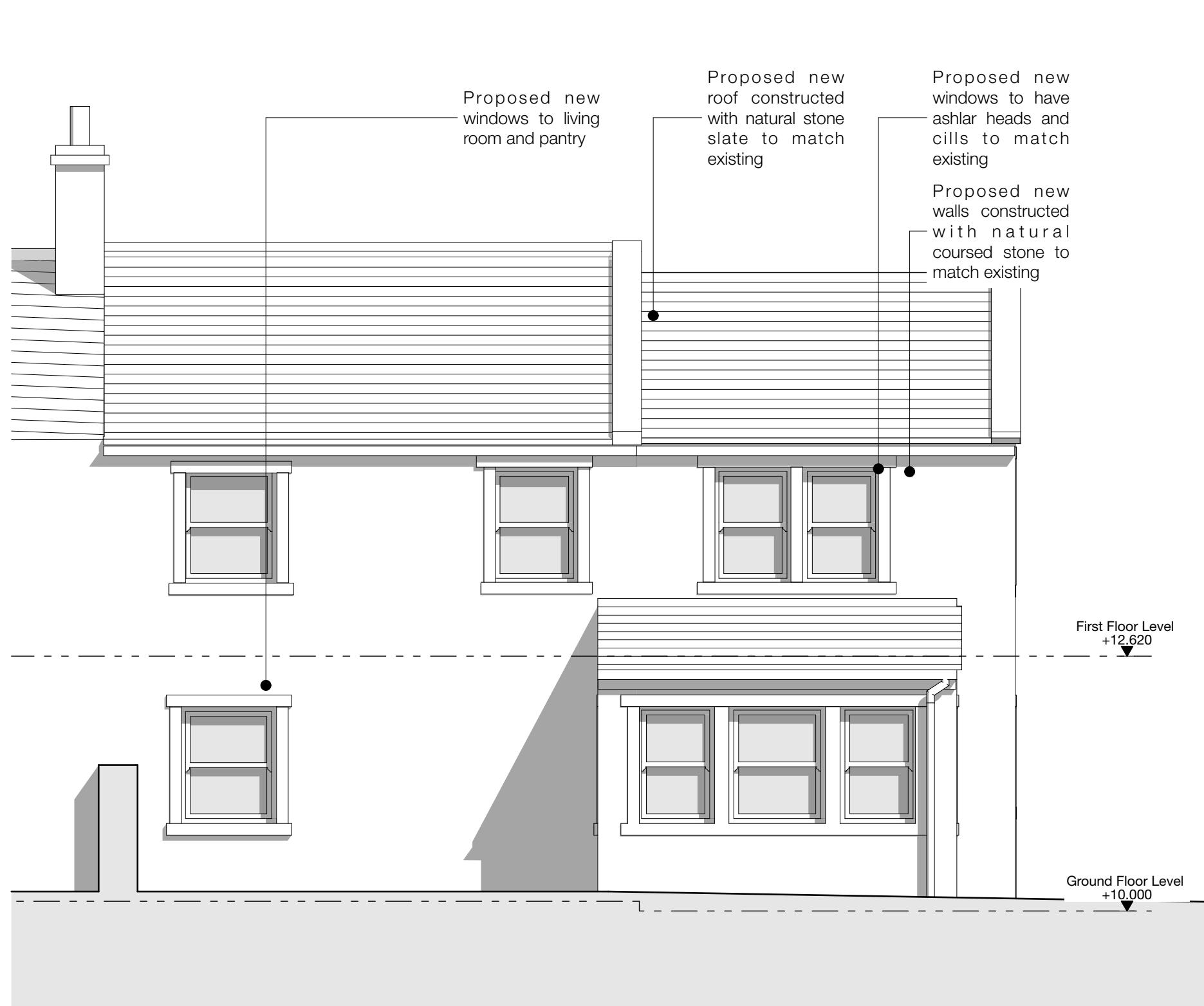
South Elevation - 1:50
