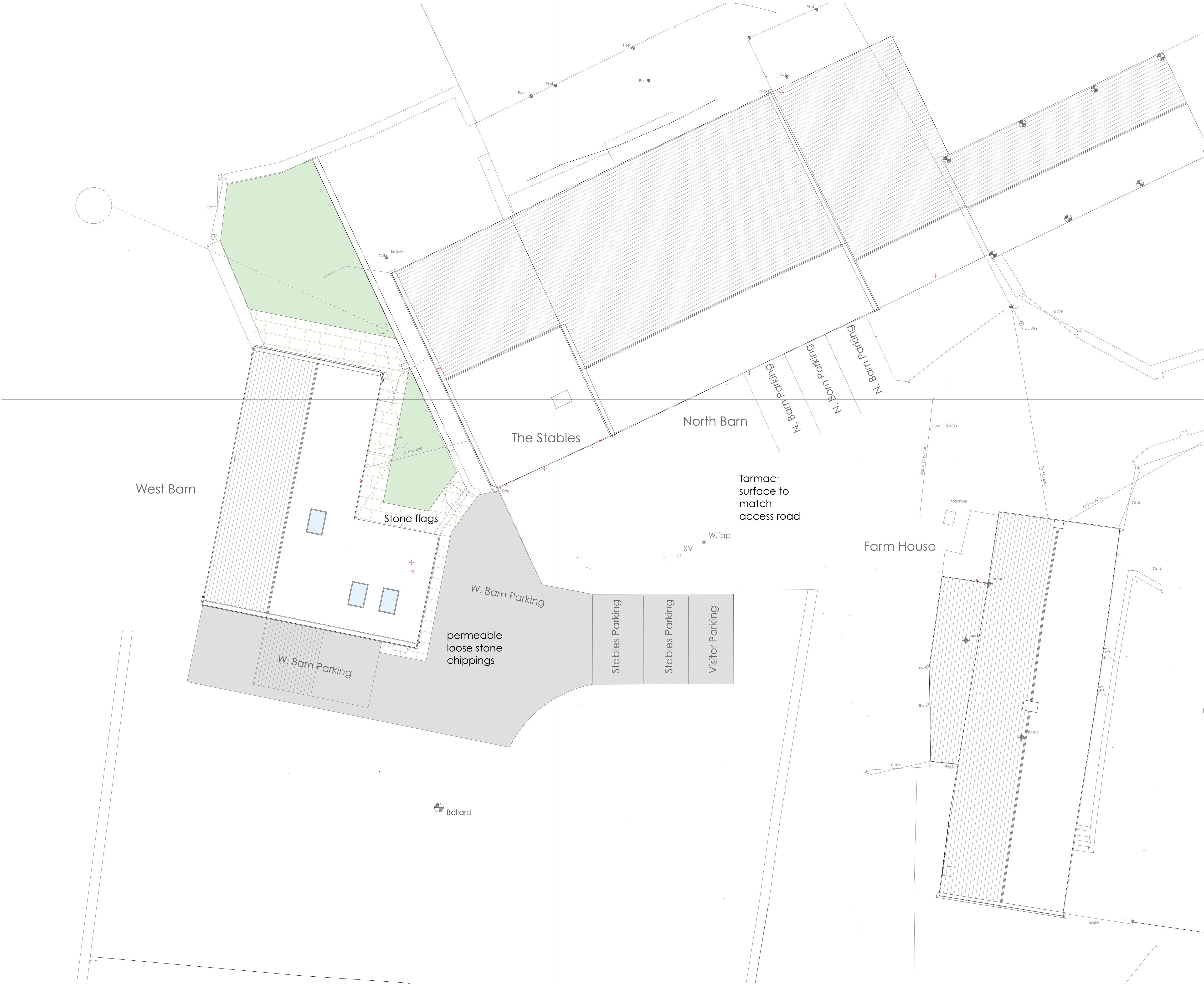
Site Plan - Parking Surfacing
