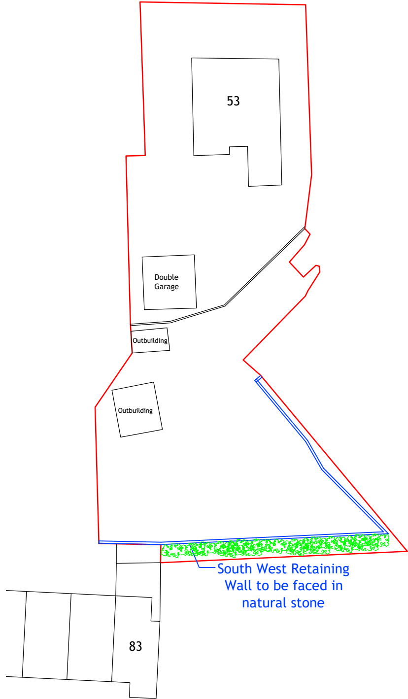
Site Layout with Retaining Wall 1.500
