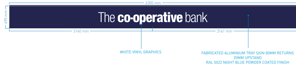
PROPOSED SHOP FRONT ELEVATION
