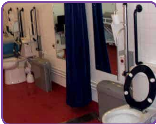
Keighley Leisure Centre's 23 sq m facilities are large enough to include two peninsular layout WCs with a privacy screen, enabling more efficient use by a visiting group
