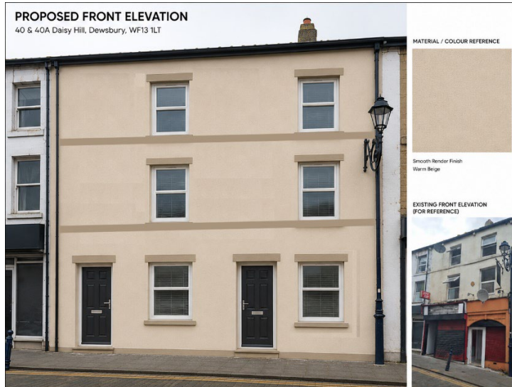
Figure 3: Proposed front elevation illustrating the removal of the existing roller shutters, installation of two entrance doors and two ground floor windows aligned with the upper-floor openings, and the application of a smooth warm beige render finish across the principal elevation.
