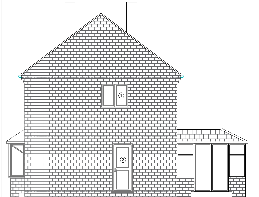
EXISTING SIDE ELEVATION (North East)
