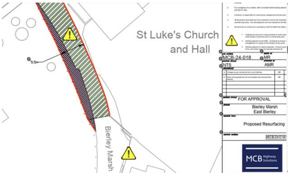
Access-Resurfacing Plan MCB-24-018
