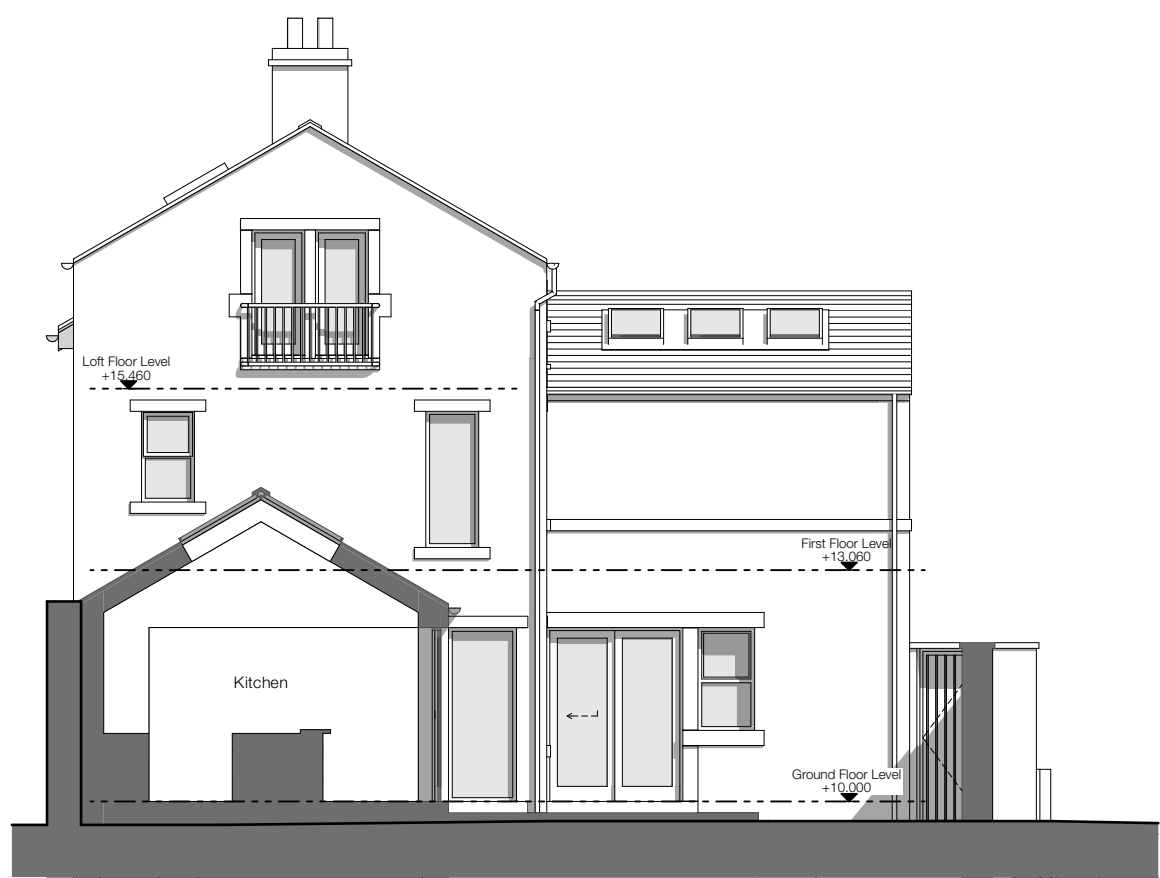
Proposed South Elevation - 1:100
