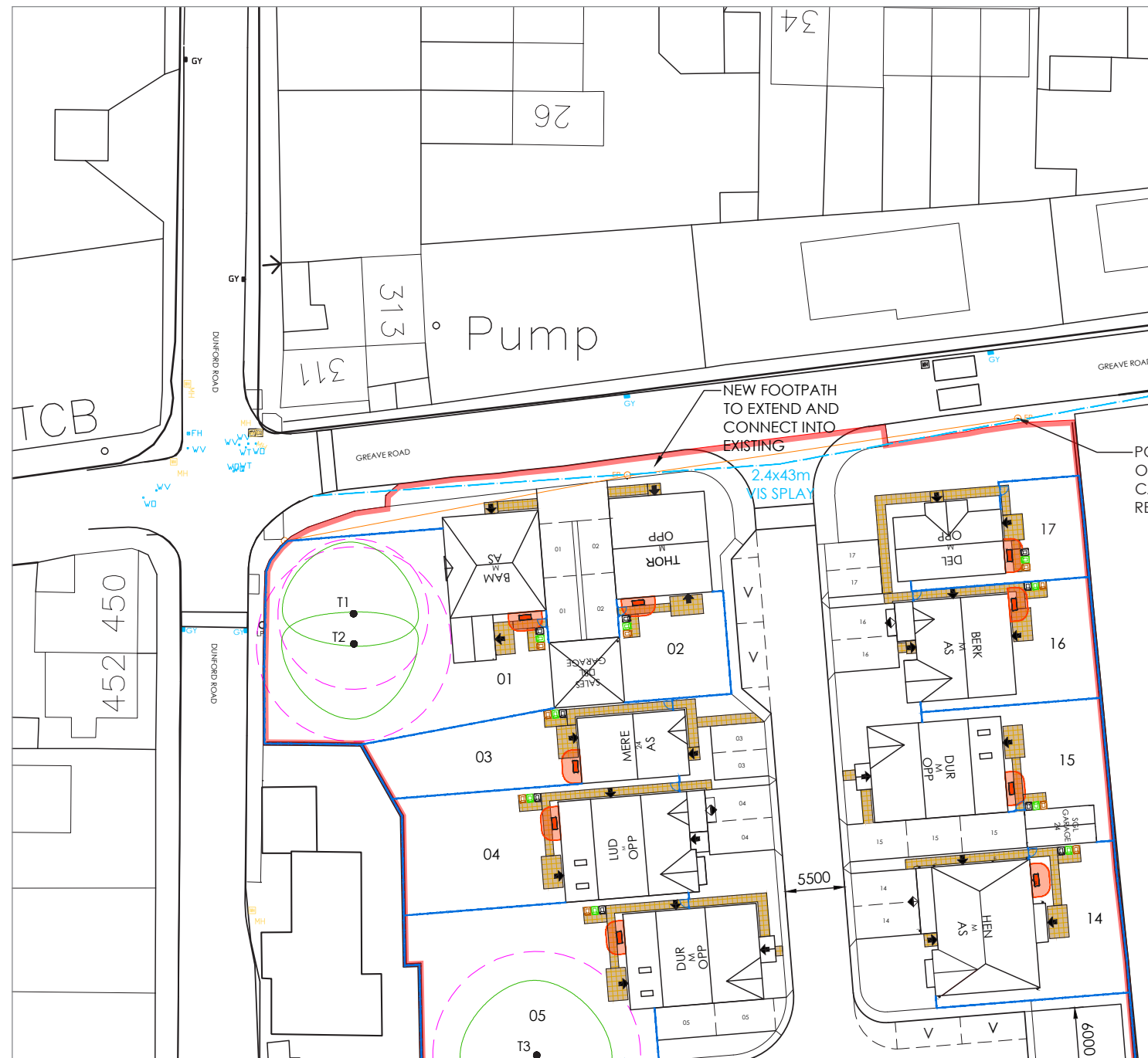
Proposed Site Layout Access Detail
