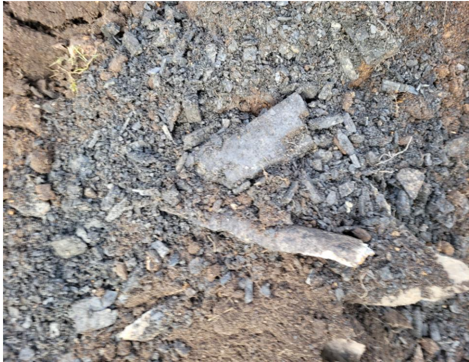
Close up of Made Ground in TP12, including the Asbestos Cement Sheetting
