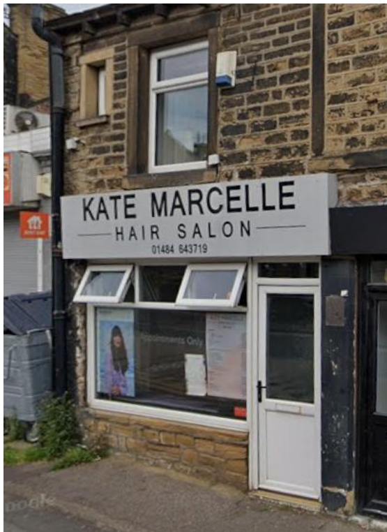
9a New Street, red rectangle is the new proposed position, The sign will be mechanically fixed to the masonry using screws/bolts into wall anchors, via a hidden backing frame, giving it a clean, flush appearance.
