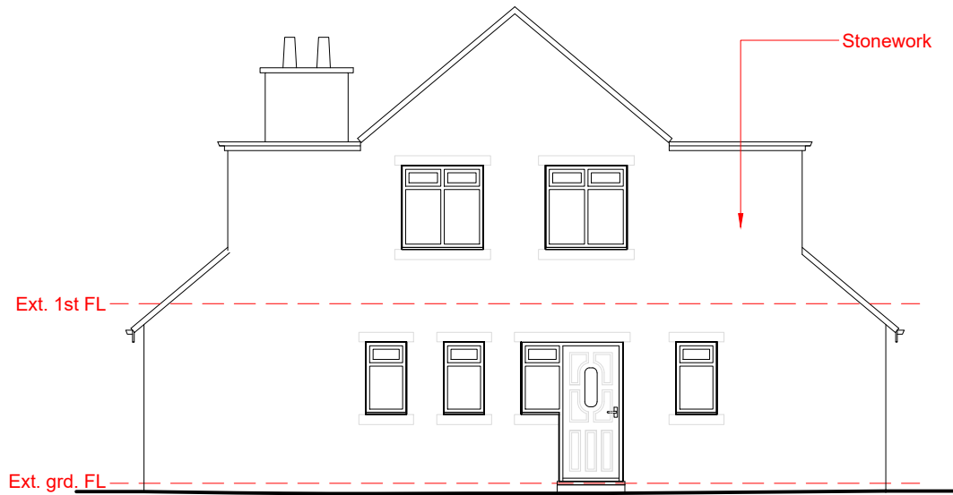
EXISTING PART SIDE ELEVATION (B)
