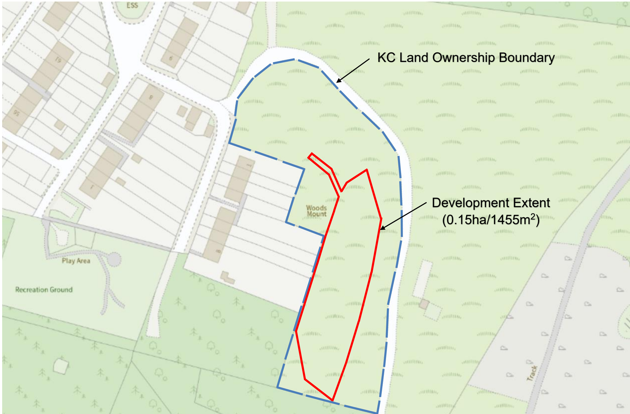
Woods Mount Flood Alleviation Scheme – Bund Earthworks and Minor Drainage – Land ownership Boundary and Development Boundary
