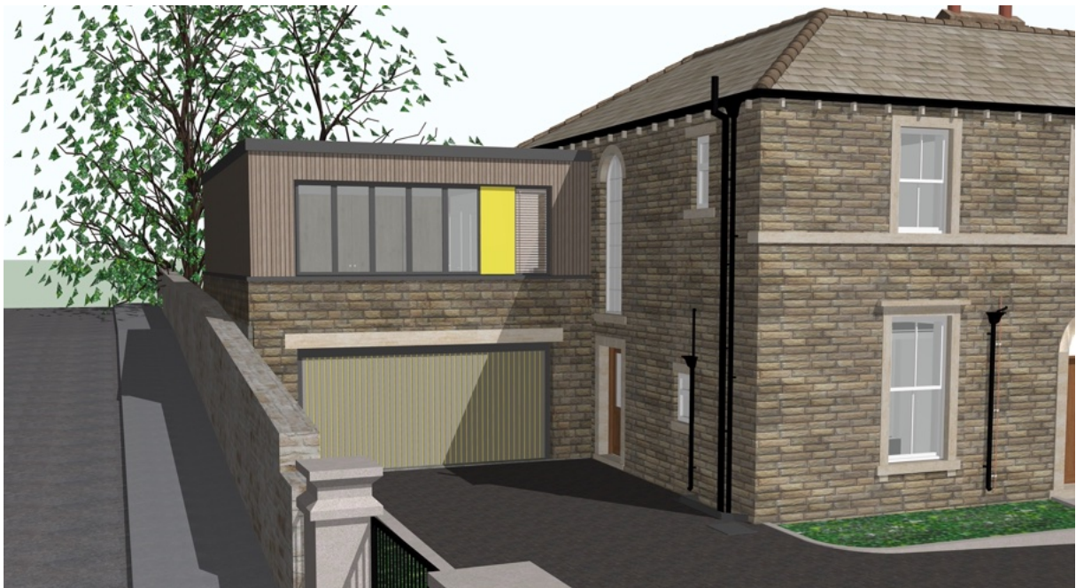
Front Elevation as proposed with vertical timber cladding over existing natural stone
