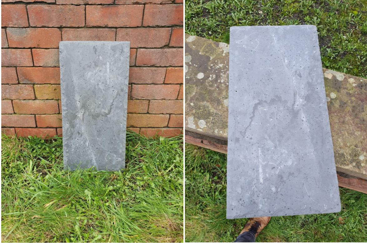
Above: The slate to be used are blue Spanish slate that also match the surrounding area. The roofing slates are a certified A1-S1-T1 product that present a smooth surface, fettled edge and uniformity in thickness. Dimensions – 500 × 250.
