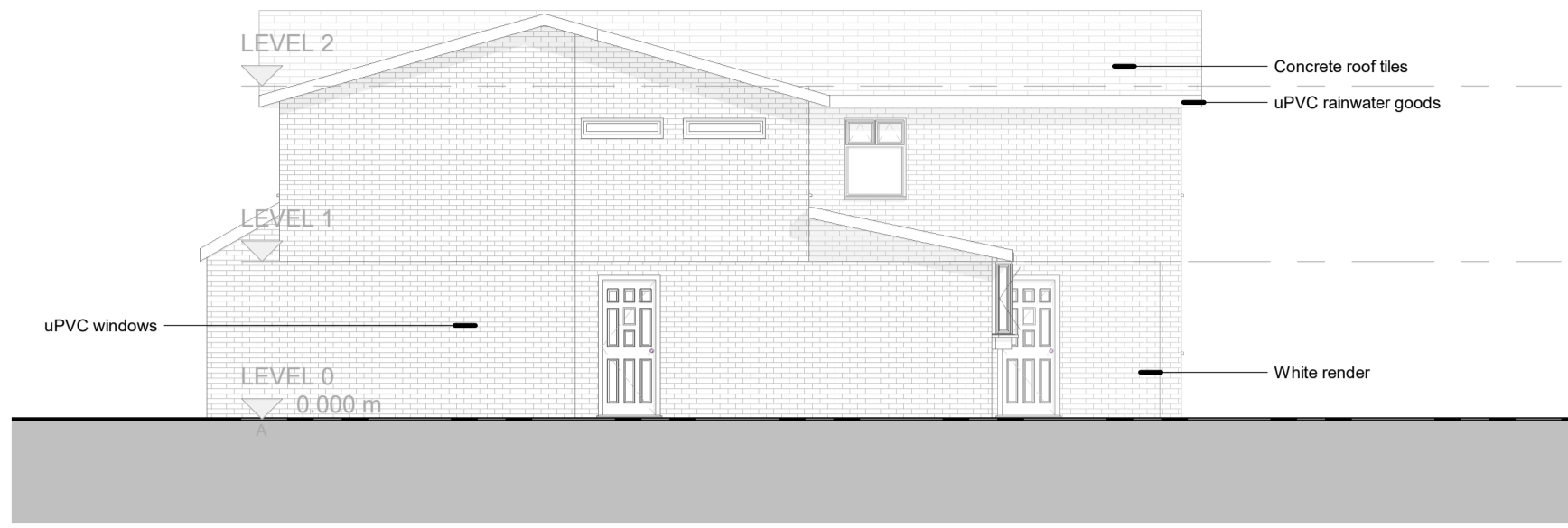
1 Existing South Elevation 1 : 100
