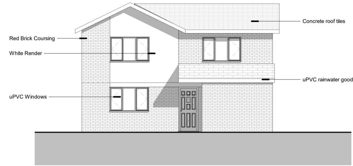
3 Existing East Elevation 1 : 100
