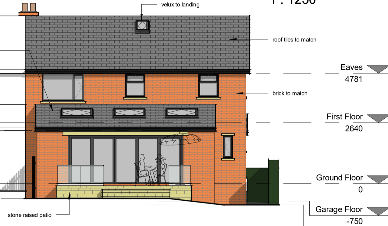
Rear Elevation (South Facing) 1 : 100
