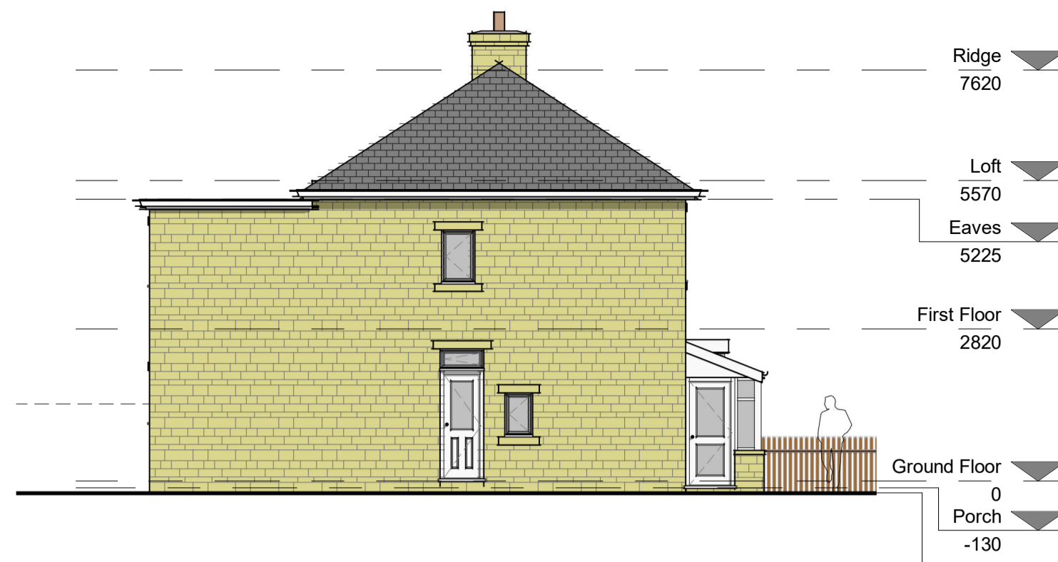
Side Elevation (SW Facing) 1 : 100
