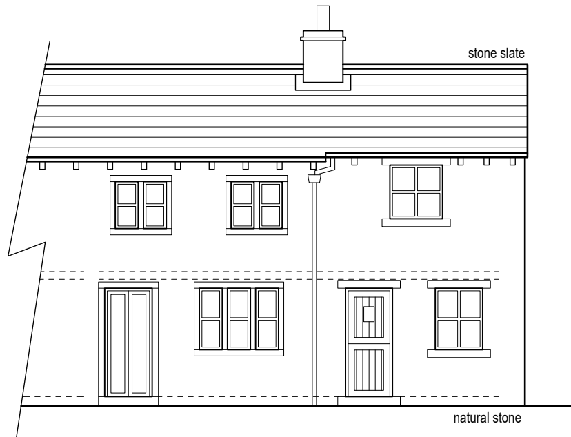
Existing front/south west facing elevation (1:100)
