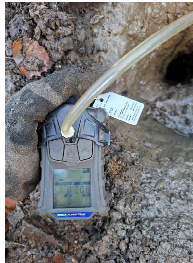
^^^ Photograph 3: Ground gas monitoring in R0101
