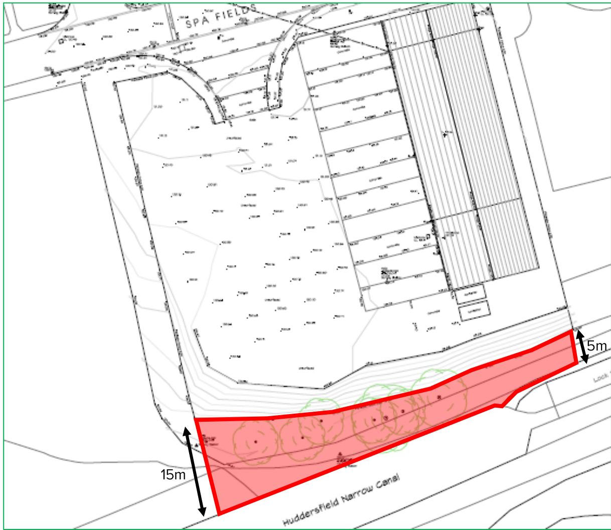
Heavy Machinery Exclusion Zone: Minimum of 5m
