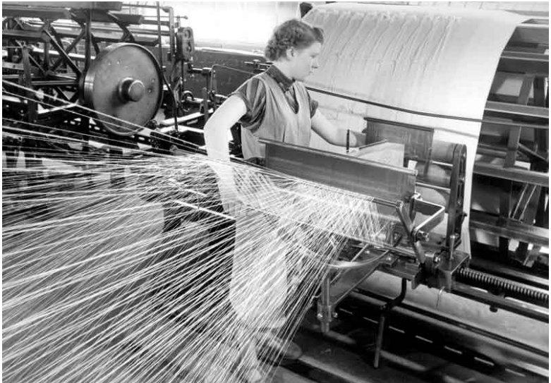
A warping machine, as would have been used at New Mills during its heyday as a working textile mill.
