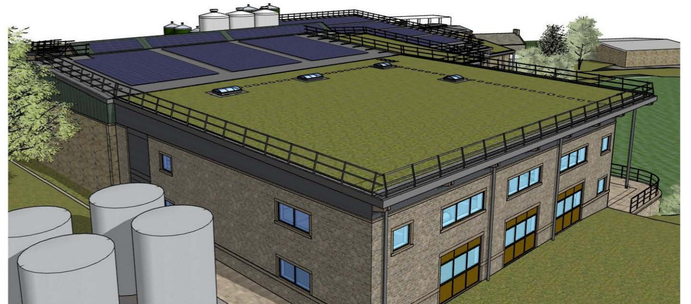
Perimeter handrails around roof edge
