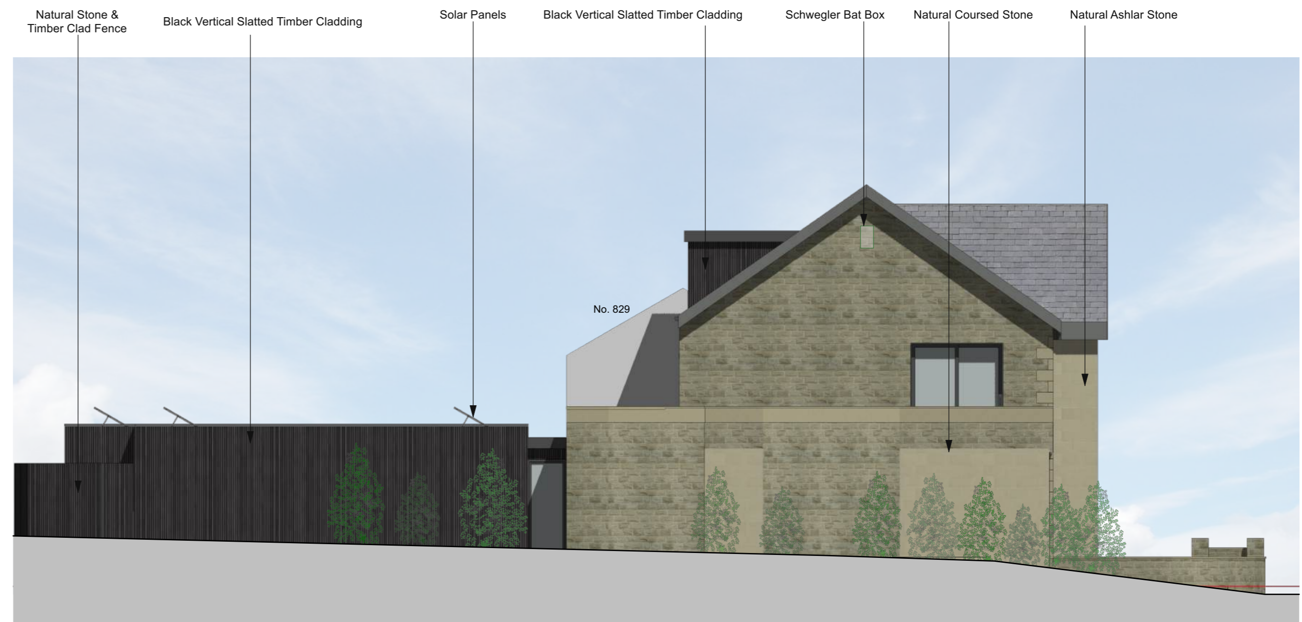
Side Elevation As Proposed Scale 1:100
