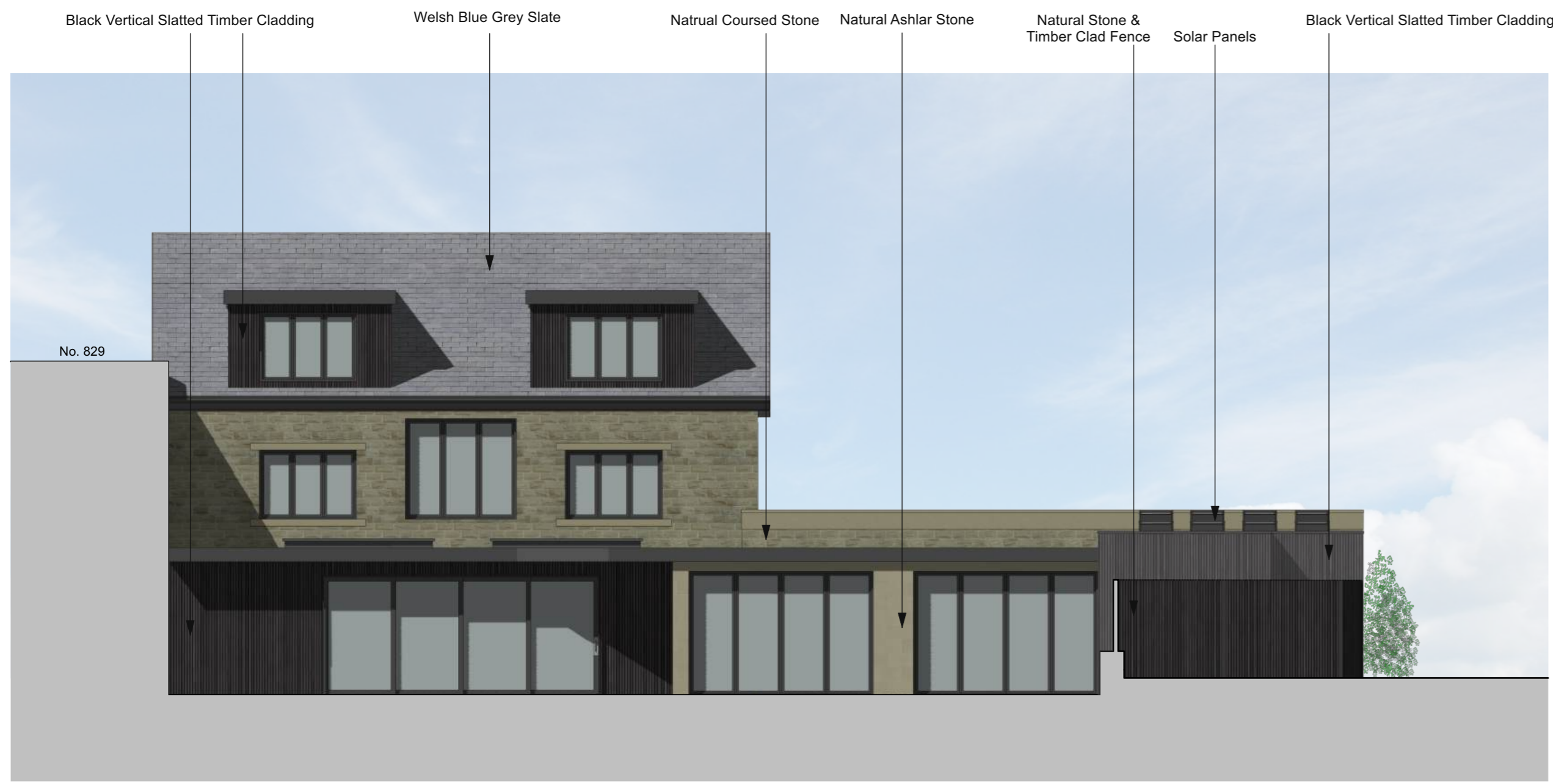
Rear Elevation As Proposed Scale 1:100
