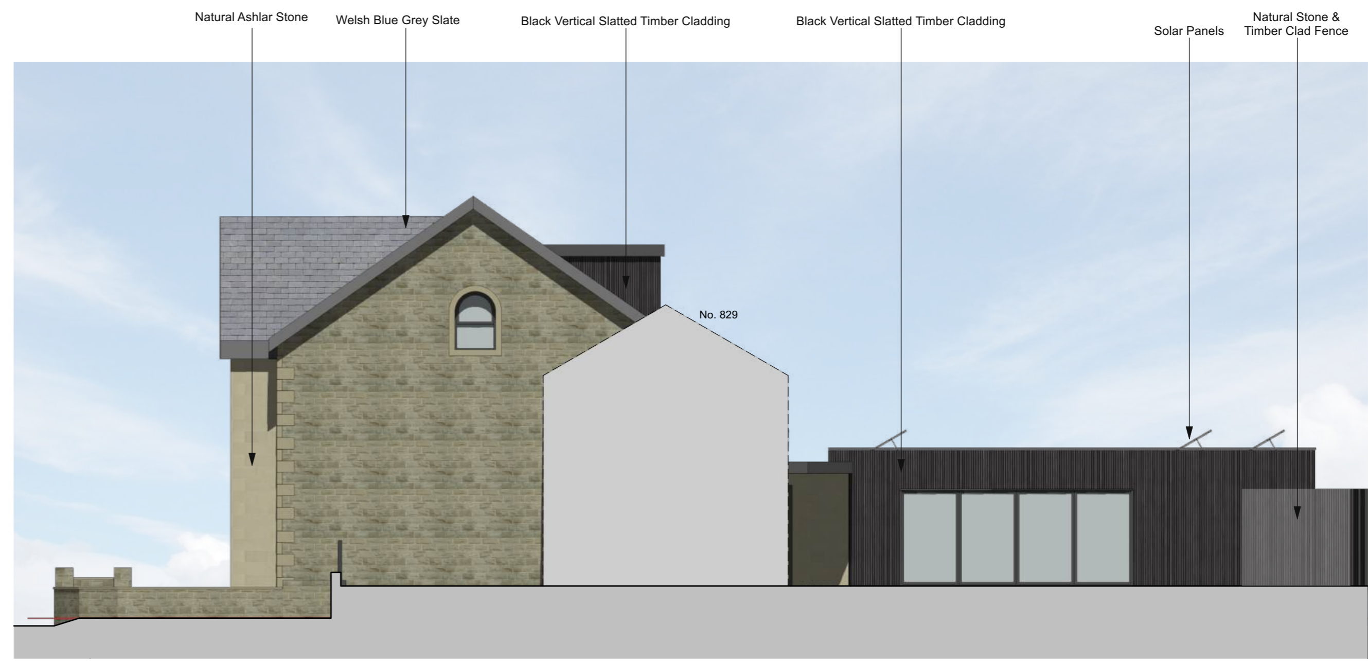
Side Elevation As Proposed Scale 1:100
