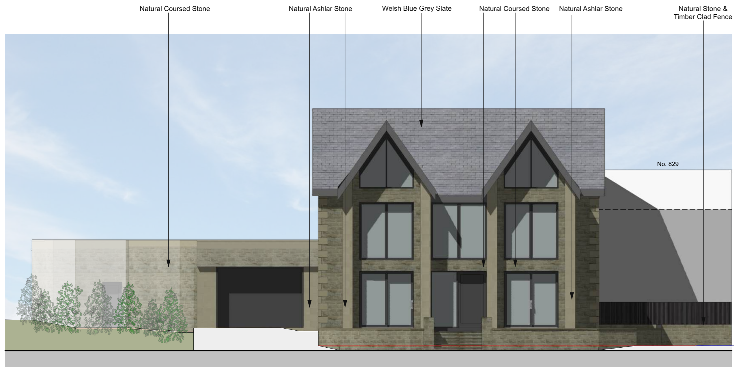
Front Elevation As Proposed Scale 1:100
