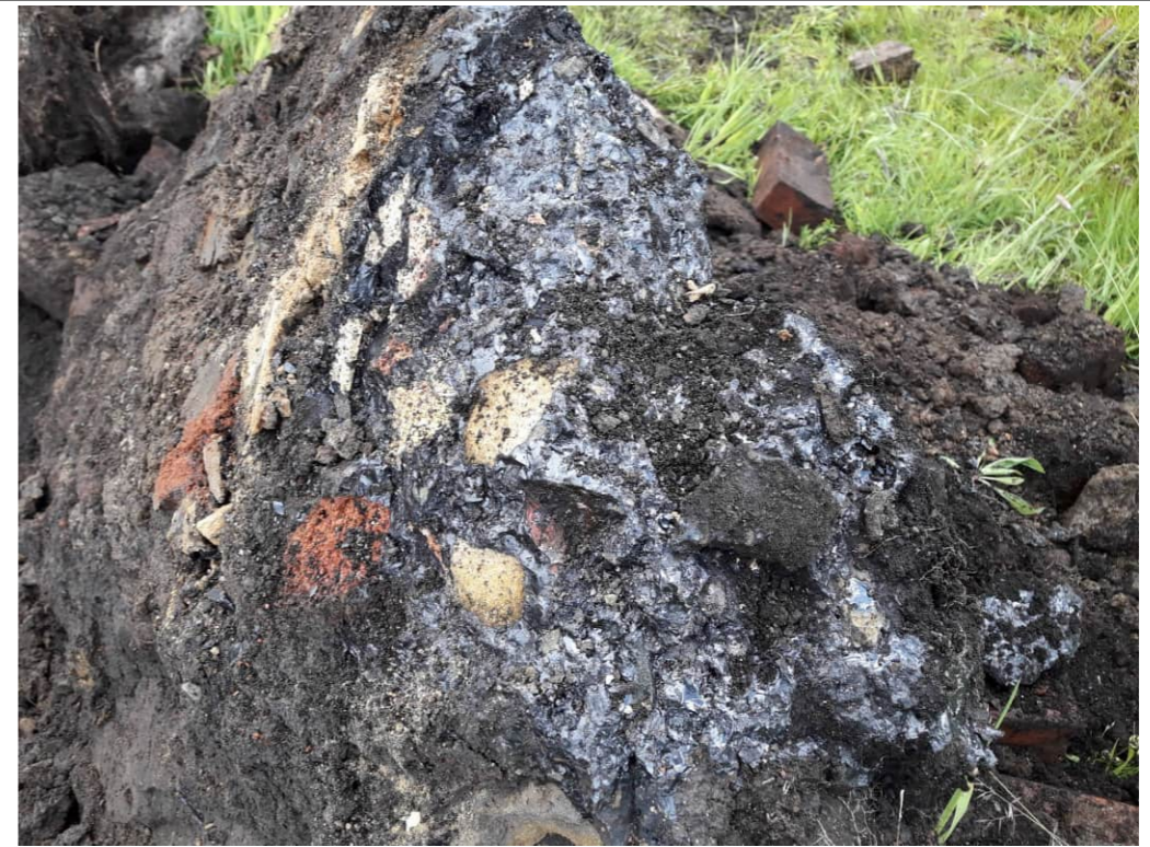
Photo 2: Bound macadam material recovered in TP06A.
