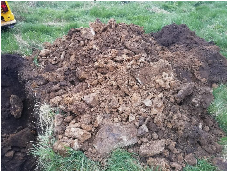
Figure 4: Trial Pit 1 Spoil
