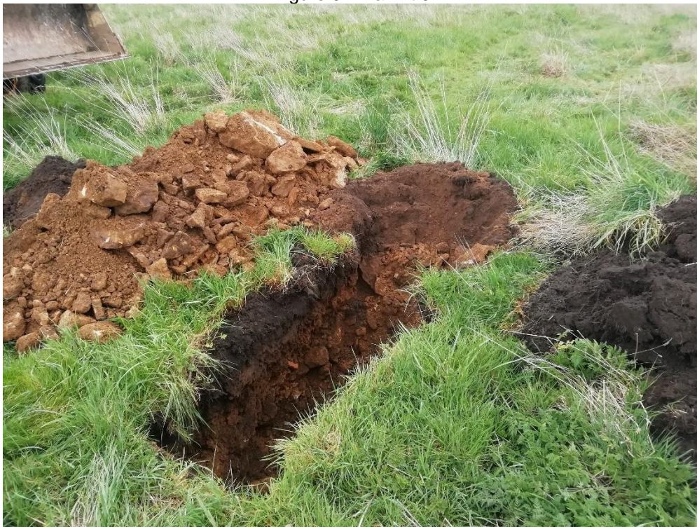
Figure 10: Trial Pit 5 Spoil
